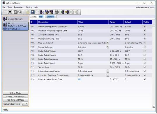
In Optitools Studio, ensure communication is established with the connected drive.
