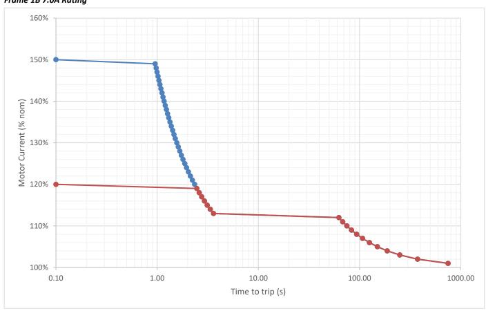
Allowed overload when heatsink temperature <60C
